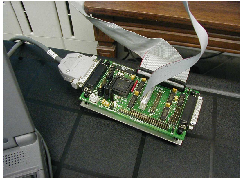
Mx1000 BTR With Serial Cable (left DB25), 50 Conductor Fanuc Tape Reader Cable (top right) and Facit 4070 Punch cable (middle). Note power for unit comes from Fanuc Tape Reader cable – truly plug and play.
