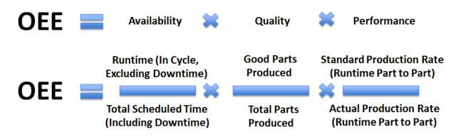
Customers who have implemented OEE utilizing MTConnect typically experience an **increase in Capacity Utilization (CU)** of 30% plant-wide, a minimum increase of 11% and a maximum increase of 110%. The tracking of OEE has a considerable financial impact in that a 10% increase in CU generates a 21% increase in Income From Operations ("IFO"). IFO is defined as operating income, EBITDA. An example is shown in the figure below.
